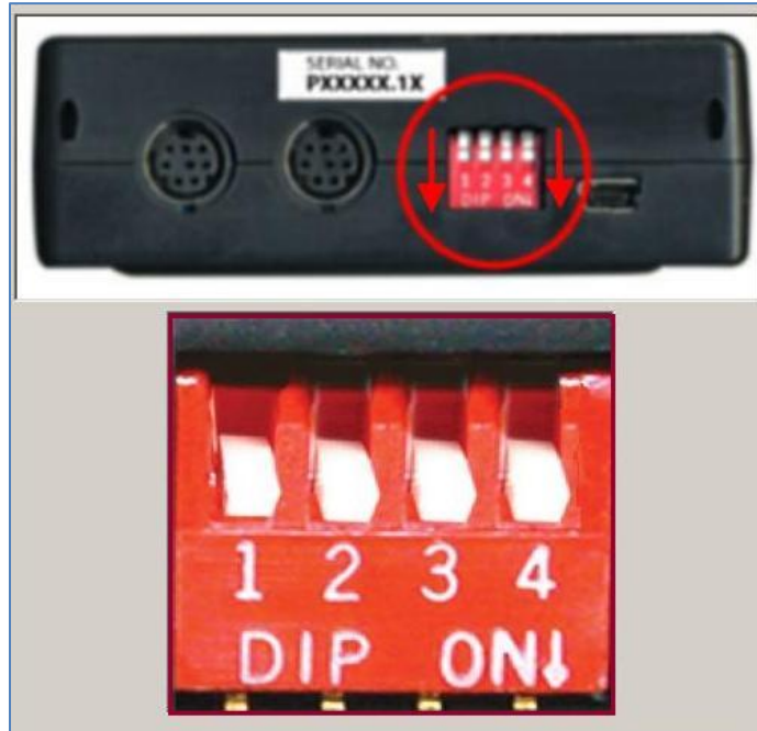
Figure 1: DIP Switches in the Down Position:
